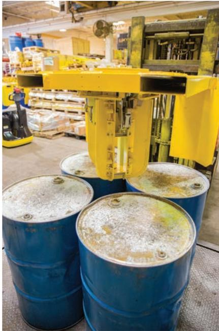
Liftomatic Material Handling, Inc. now offers attachments to handle up to four drums at once. It is selling two forklift-mounted attachments suited for high-volume drum handling.
