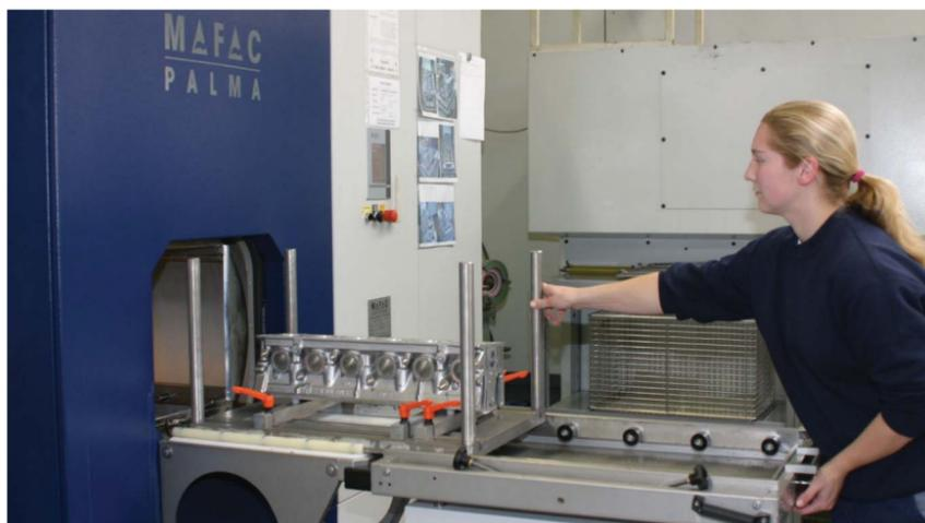
Wet chemical cleaning of individual parts can be used in order to assure that required levels of cleanliness are complied with for workpieces with complex geometries. It allows for targeted treatment of channels, drill-holes and undercuts.
