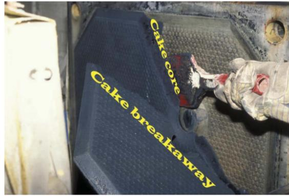
that there is much less volume to transport and the sludge is in a cake phase. Typically this is accomplished by conditioning the sludge with a chemical agent - such as a polymer - to help the sludge particulate release its water phase. The conditioned sludge is then run across a centrifuge, a belt filter press or a pressure filter to remove the water and provide the cake. In general, the drier sludge comes from the pressure filter with less
