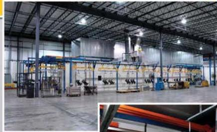
A SlideRail Square Transfer™ (SST) electrocoating system not only fit into their building, it offered a second color option down the road. The SST handles both steel and aluminum substrates and included reverse osmosis, iron removal and wastewater treatment equipment.
